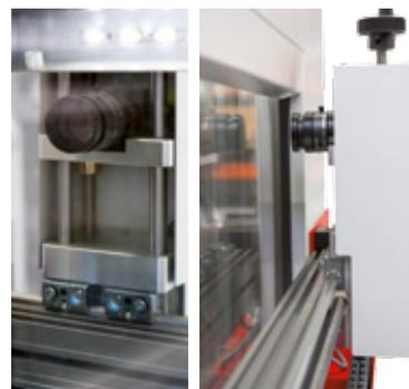
CCD Camera system for crack-growth measurement
