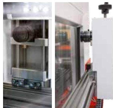
CCD Camera system for crack-growth measurement
