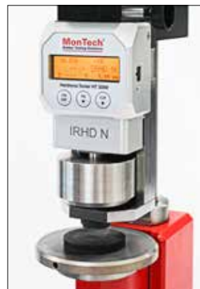
IRHD Normal measurement on parts
