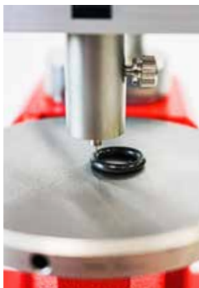
IRHD Micro measurement on O-Rings
