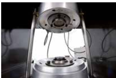
Die upgrades including precision heaters and probes
