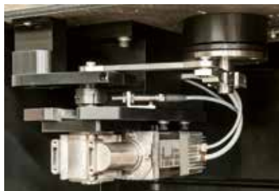
Rheometer brushless DC drive upgrade
