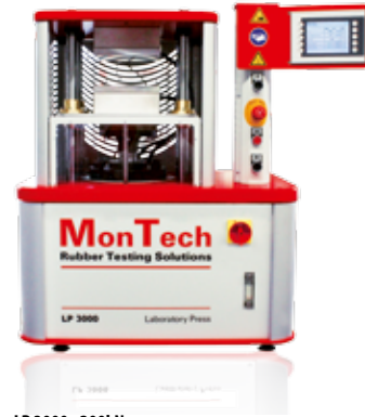
LP 3000 - 200kN Medium size benchtop hydraulic laboratory press
