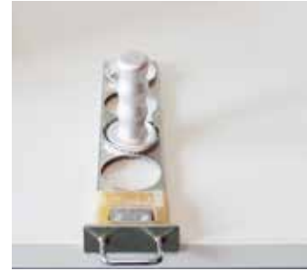
3 - Install aluminum dish
