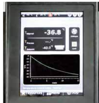
Sample temperature recording by optional immersion probe
