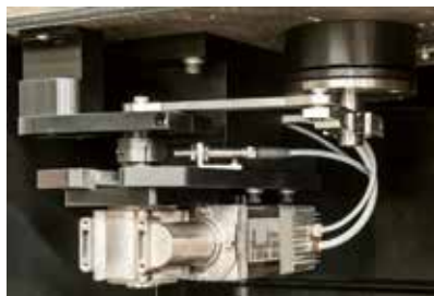
Rheometer brushless DC drive upgrade
