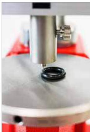
IRHD Micro measurement on O-Rings
