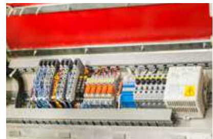
Advanced, PLC based control and DAQ electronics
