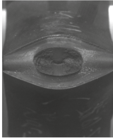
Crack growth after 100.000 samples at 60°C
