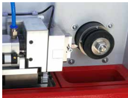
Closed loop controlled cut and chip actuator with multi-axial force sensor
