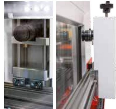
CCD Camera system for crack-growth measurement
