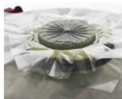
SBR Polymer sample after Mooney viscosity testing. Various types of testing film are available for easy sample handling, reduced cleaning needs, less die contamination and therefore improved repeatability.
